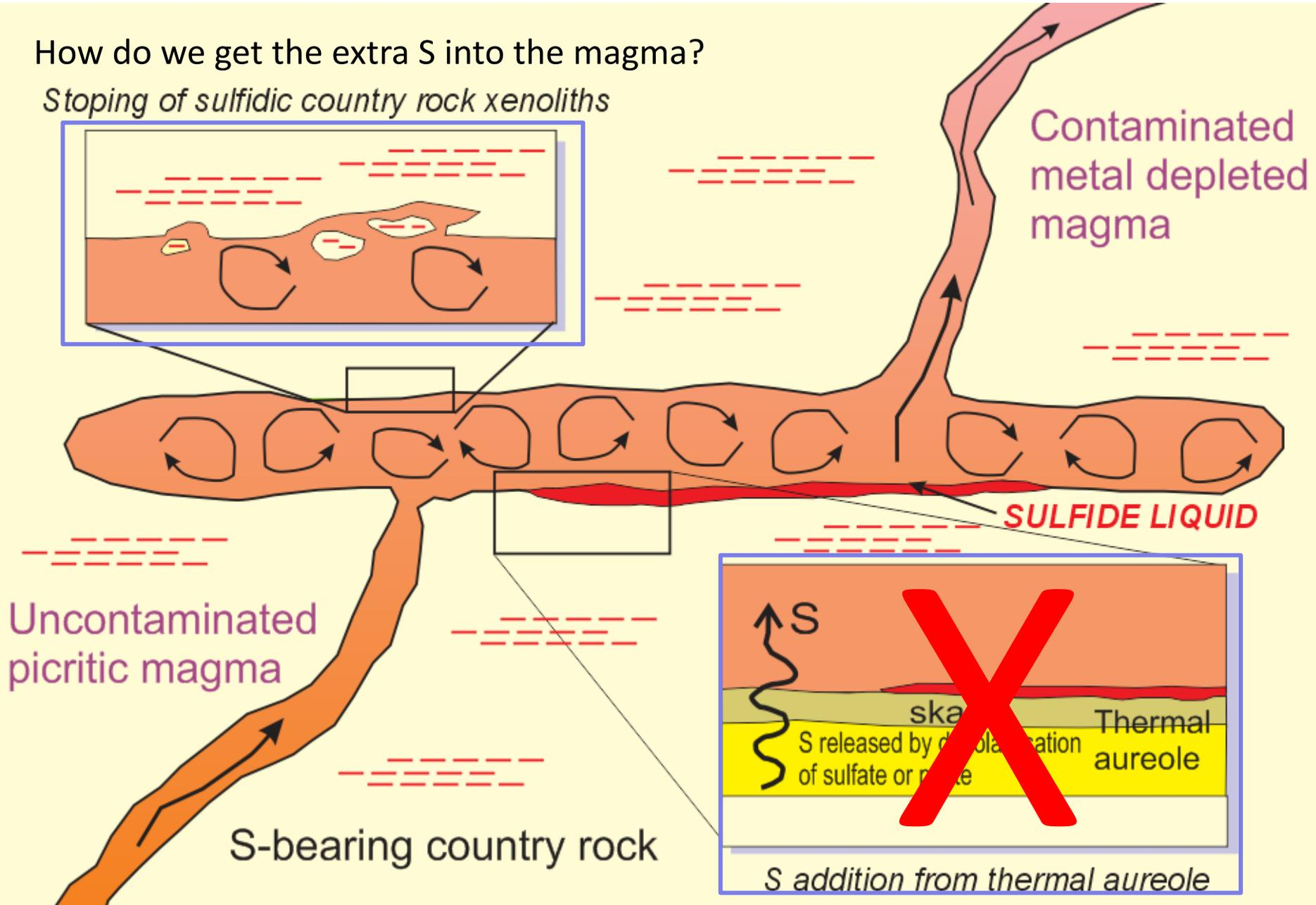
Stopping of sulfidic country rock xenoliths
