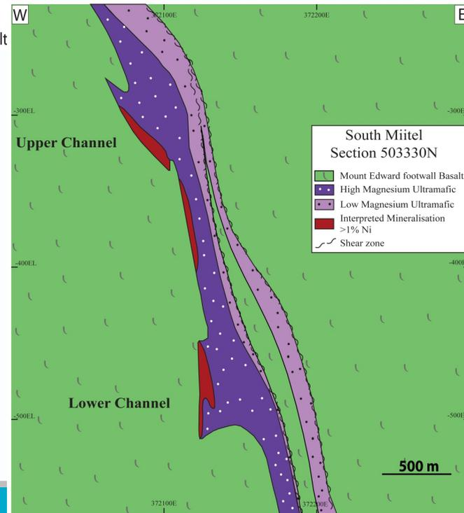
Troughs and channels due to thermal erosion
